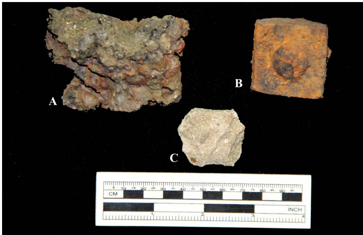
Figure 5.42. Slag (A), large square nut with a possible portion of a bolt inside the threading (B), mortar sample (C) from Site 16SBJ74 in Railroad Tie-in Survey area.
